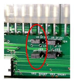
And this is the same thing for the expansion connector pin #24 with the "Digital Frequency Input 3. The expansion connector pin #23 named "VR DFIN3 –" is normally connected to the second wire of the VR sensor.
