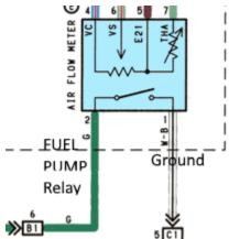
We suggest to control the fuel pump with the MS3Pro. To do that, connect green wire #2 to and spare output like INJJ on the expansion connector (pin 17).
